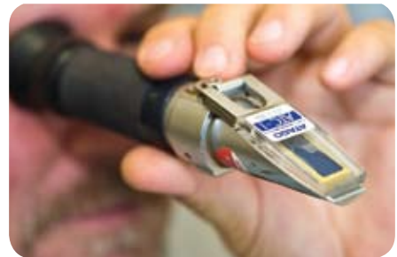
Direct the refractometer to a good light source.
